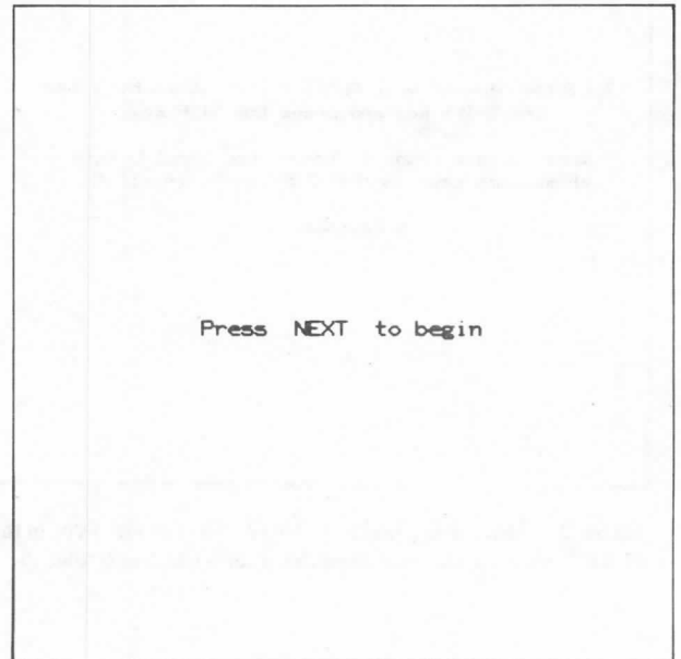
Figure 2-1. Sign-on Sequence: "Press NEXT to Begin". Either the display shown here or the display in Figure 2 should be the first you will see at the terminal. If there is something else on the display screen, press the "SHIFT" key and the "STOP" key (SHIFT-STOP) together several times until this display appears.
