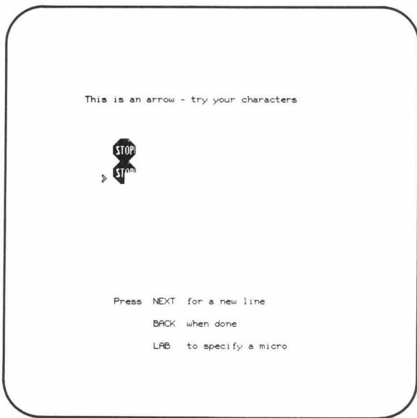
Complete and partial stop signs are constructed of pieces from the full character set. (Lisa Parker)
